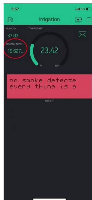
Fig.9: Ultra Sonic sensor reading in Blynk App on mobile Phone focusing on the ultrasonic reading
