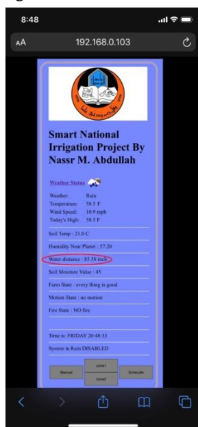
Fig.8: GUI designed by the authors for the national smart irrigation system focusing on the ultrasonic sensor readings
